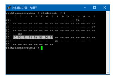
The EEPROM can be accessed for read/write operations using i2c-tools utilities, such as i2cdump
