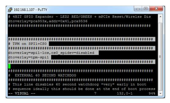
This configures SPI-1 interface and the TPM, when the system has booted it will create a /dev/tpm0 node.
