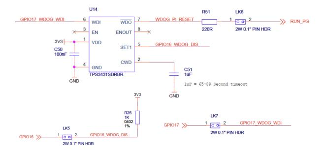
Once the watchdog is enabled the WD Input pin on the device must be togged H-L-H at least once per watchdog time-out period (60 seconds) and the low level pulse period must be >1uS long for the transition to be valid.
