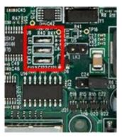
The external watchdog device is driven by GPIO29 (/WD Enable) and GPIO28 (/WD Input), by default the watchdog is disabled as GPIO29 is pulled high by default pin state.
