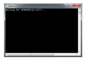
Power up the unit and RPi-Boot will configure the unit to appear as a flash drive :
