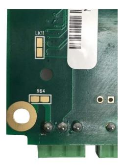
The connection of R64 is dependent on the enclosure design and how the overall chassis ground is delt with at a system level.
